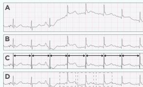
Data preprocessing. Raw data (A) was high-pass filtered (B). R-R intervals were calculated (C), and 1.5 second 3-beat trains were extracted.
